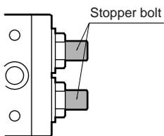
**8** Observe steps (1) to (5) when adjusting the angle. If the angle is not adjusted this way, the seal washer may break after one or two adjustments.
