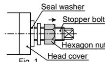
(2) Separate the seal washer from the head cover as shown in Fig. 2.
