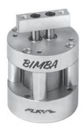
Flat-II nonrotating, double-acting cylinder provides the answer to applications where rotation cannot be tolerated and space is at a minimum. Nonrotation is achieved with dual piston rods and a rod end block that insures the rods work in tandem. Flat-II eliminates the need for external alignment devices, such as guides, rods and alignment posts or pins.
