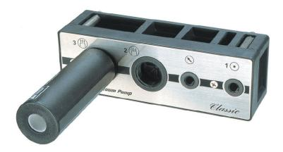
A traditional Piab vacuum pump developed to be used within the chemical industry or in chemically aggressive environments. It can achieve higher vacuum levels, even down to 100.8 -kPa. It is available with connection plate in composite PPS or aluminium. We recommend it to be used with practically zero leakage present and in nonporous applications.
