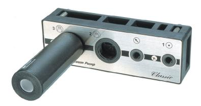
A traditional Piab vacuum pump developed to be used within the chemical industry or in chemically aggressive environments. It can achieve higher vacuum levels, even down to 99.8 -kPa. It is available with connection plate in composite PPS. We recommend it to be used with practically zero leakage present and in nonporous applications.
