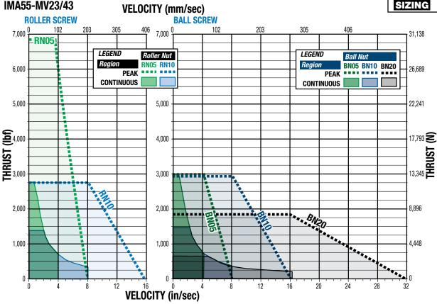
PEAK REGION is the maximum performance capabilities of the actuator system. Higher peak thrusts are achievable by servo motor actuator systems, so please consult Tolomatic before exceeding catalog rating.
