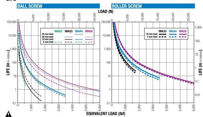
NOTE: The  $\mathbf{L_{10}}$  expected life of a ball screw linear actuator is expressed as the linear travel distance that 90% of properly maintained ball screw manufactured are expected to meet or exceed. This is not a guarantee and this graph should be used for estimation purposes only.
