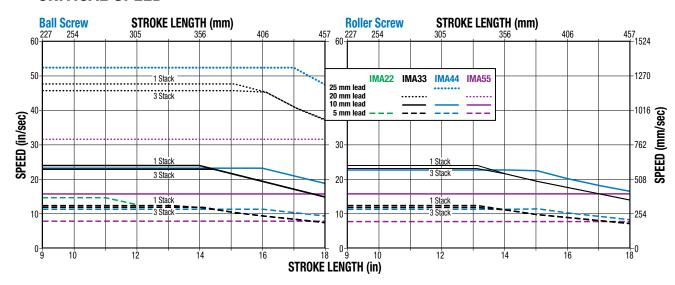
All curves represent properly lubricated and maintained actuators.
