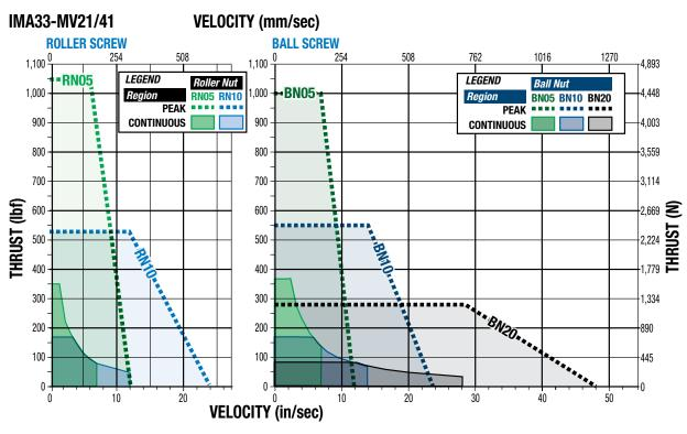
PEAK REGION is the maximum performance capabilities of the actuator system. Higher peak thrusts are achievable by servo motor actuator systems, so please consult Tolomatic before exceeding catalog rating.
