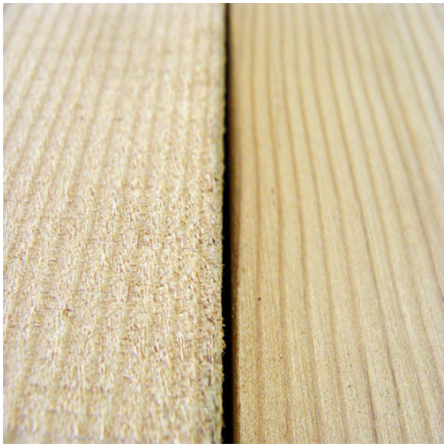
Rough and irregular lumber
