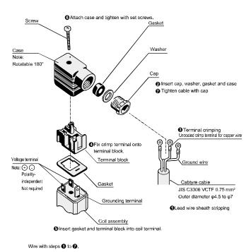
\* The orientation of the cord can be changed by removing the terminal block from the case, rotating it by 180°, and then replacing the block into the case.
