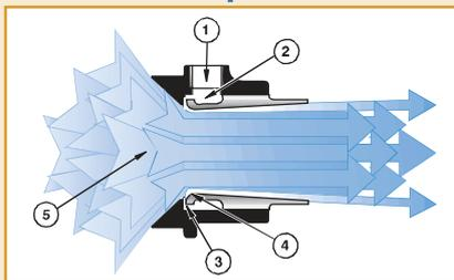
Compressed air flows through the air inlet (1) into an annular chamber (2). It is then throttled through a small ring nozzle (3) at high velocity. This primary airstream adheres to the Coanda profile (4), which directs it toward the outlet. A low pressure area is created at the center (5), inducing a high volume flow of surrounding air into the primary airstream. The combined flow of primary and surrounding air exhausts from the Air Amplifier in a high volume, high velocity flow.
