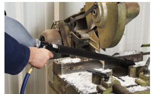
Model 6392 Vac-u-Gun All Purpose System removes plastic shavings from a saw.
