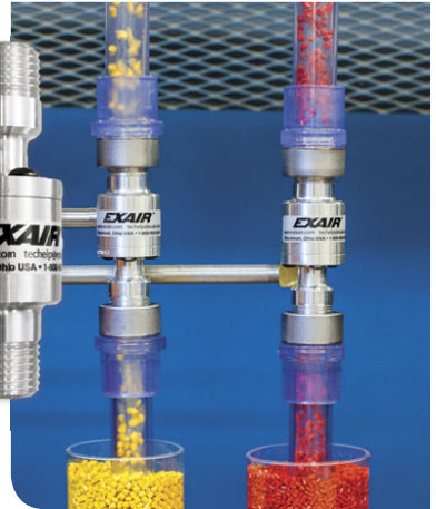
Plastic color concentrate pellets are added to a plastic extrusion process.
