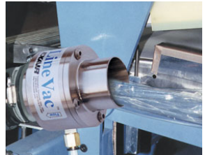
A Model 6084 2" (51mm) Line Vac transports scrap cellophane trim to a waste barrel.
