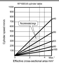
This cylinder table shows the available range according to the air supply and exhaust flow rate of the precision regulator and the required consumption flow rate at the cylinder PUSH/PULL.
